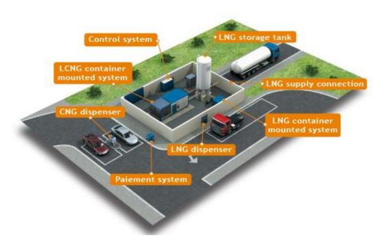
Figure 2.3: Typical Plant layout for LCNG & CNG Filling Station
