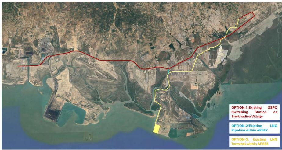
Figure 6-1: Alignment Routes for laying of NG Pipeline
