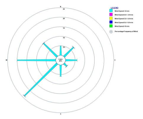
Figure 3.6: Windrose Diagram (From) for Day
