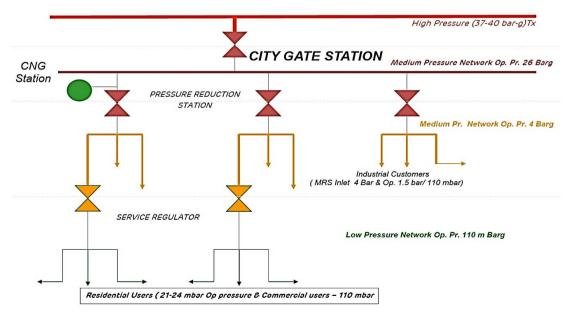
Figure 2.2: Network Conceptual Plan as per Pressure Regime
