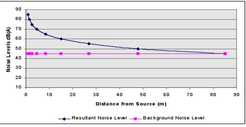
Figure 4.1: Attenuation of Noise Levels
