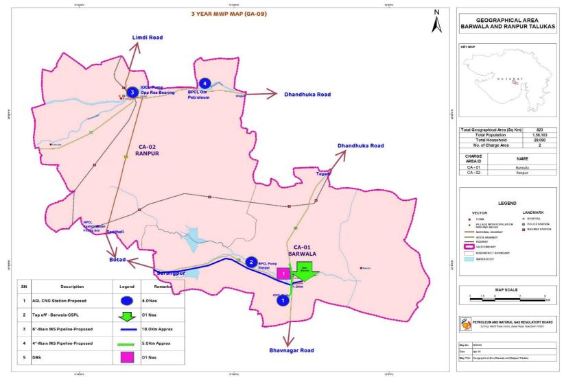
Figure 2.3: Pipeline Route, Locations of DRS and CNG Stations
